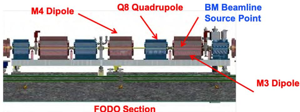
*Figure 3.21. An elevation view of the BM source location in the FODO section.*
